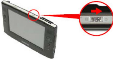
Make sure that you switch the Power switch to the **right**, NOT to the left, if you want to turn on the computer. Switching it to the left will launch AVStation Now, of which the meaning is irrelevant for your purposes, and will not switch on your computer.
