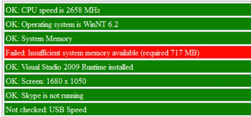
**Figure 6: Diagnosis interface - memory test failed**
