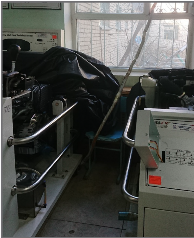
Figure 12: Diesel Engine Simulator with Improvised Exhaust Tube
